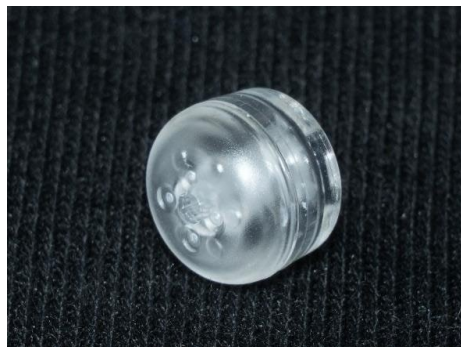
CAPDCM microfluidic implant—assembled shells designed to capture tumor cells.
