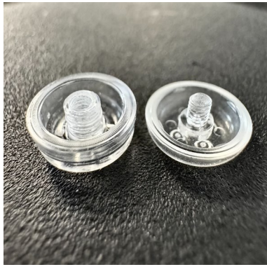
Two halves of the microfluidic implant and a top view of one half with a scale.
