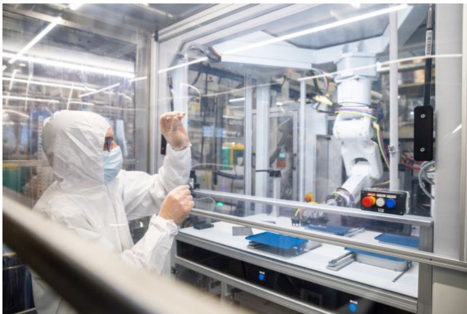
Robotic production cell in an ISO 7 cleanroom.
